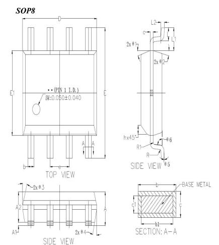
COMMON DIMENSIONS (UNITS OF MEASURE=MILLIMETER)
