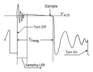
Fig.2. Voltage of Auxiliary-winding Waveform
