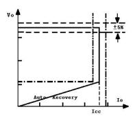
Fig.1. Typical CC/CV Curve
