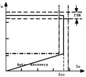
Fig.1. Typical CC/CV Curve
