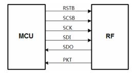
The data and control interface gives access to all the features in the chip. The data and control interface consists of the following seven digital signals:
