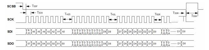
**Note:** The device SPI bus setup data when the rising edge of the master SCK, and sample data at the falling edge of the master SCK.
